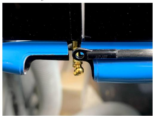
3, fit the servo mount plate rear end to the front end of wing joiner hole and mark the servo arm position on the fuselage
