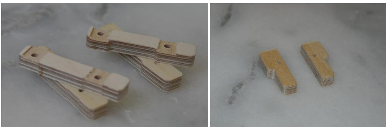
Fig. 7: Left: Servo mounting pads for Graupner DS3288 (split such that top part can be removed for servo disassembly). Right: Mounting pads for MKS DS6125.
