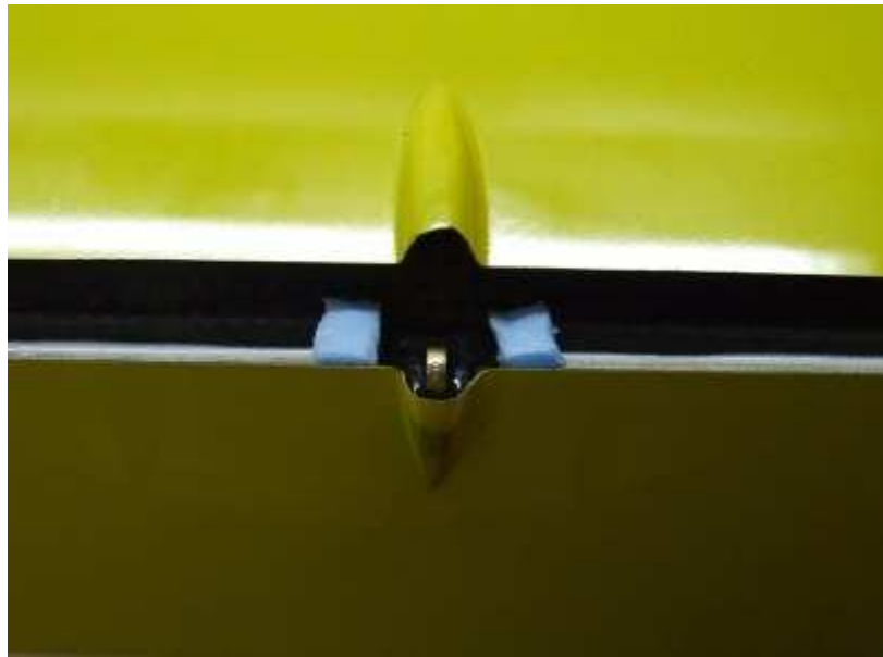
Glue horn with thickened epoxy.
