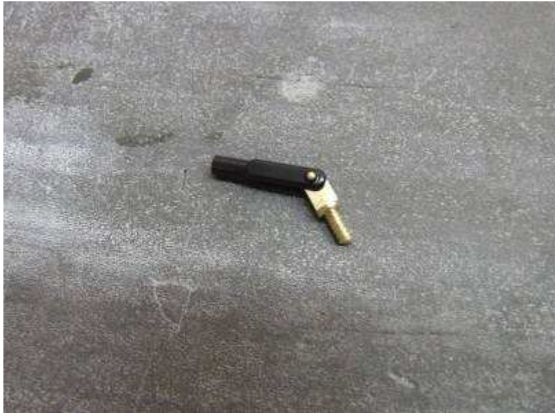
Prepare aileron horns (bevel lower end).
