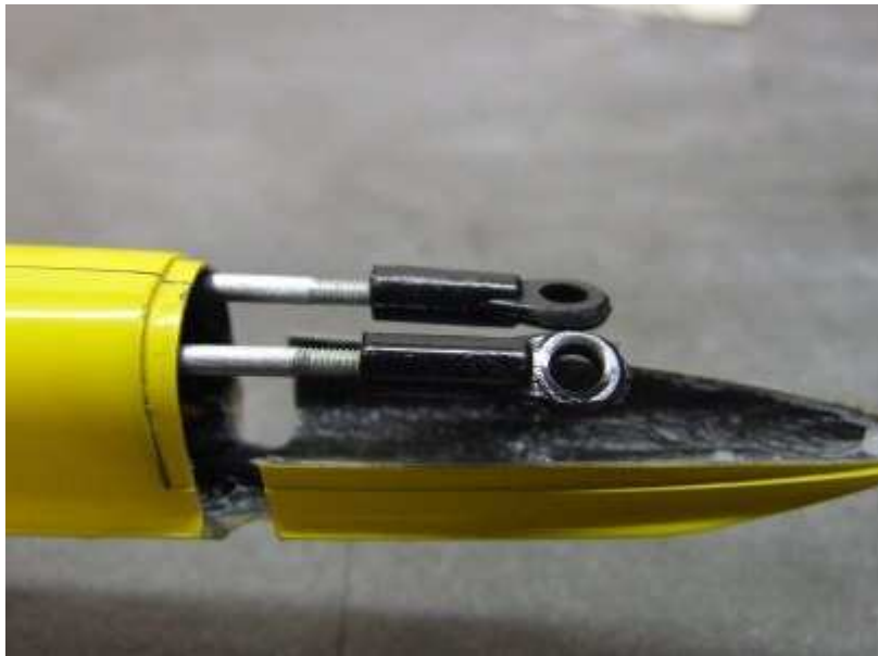
Screw the ball links to the Bowden wires.
